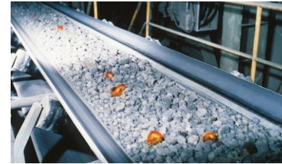
New conveyor belt which combines high-heat resistance and flame-resistance properties (image)
