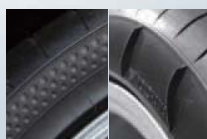
Dimpling (left) and fins arrayed on a tire to reduce air drag
