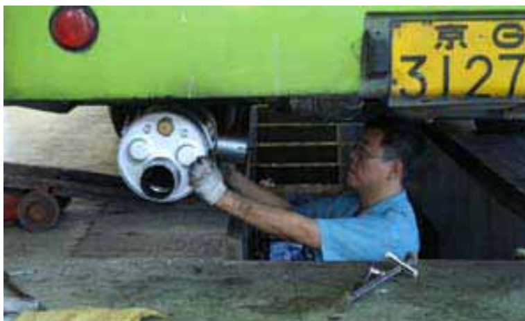
Beijing, China - Pirelli Eco Technology particulate filters
